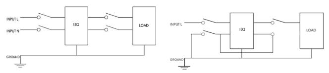
**Figure 3** – Correct Power Configuration
