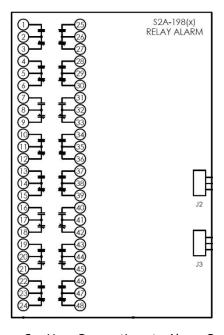
Figure 6 – User Connections to Alarm Contacts
