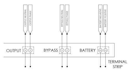
Figure 2 – Example I31 Terminals for 1-Phase Output
